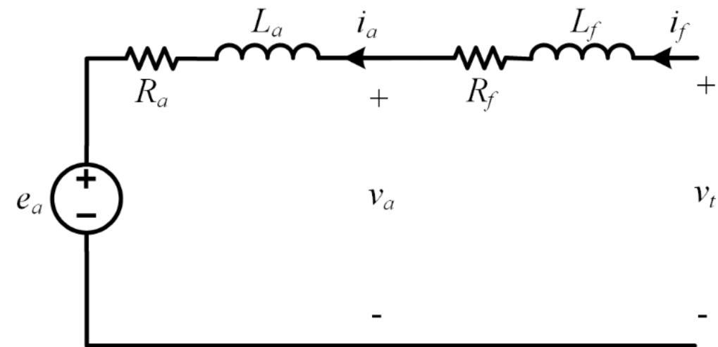
$$\begin{aligned} v_t &= (R_a + R_f) i_a + e_a; \quad e_a = K \phi_f \omega_m; \quad \phi_f = C i_f; \quad i_f = i_a \\ \Rightarrow v_t &= R i_a + K C i_a \omega_m \end{aligned}$$
