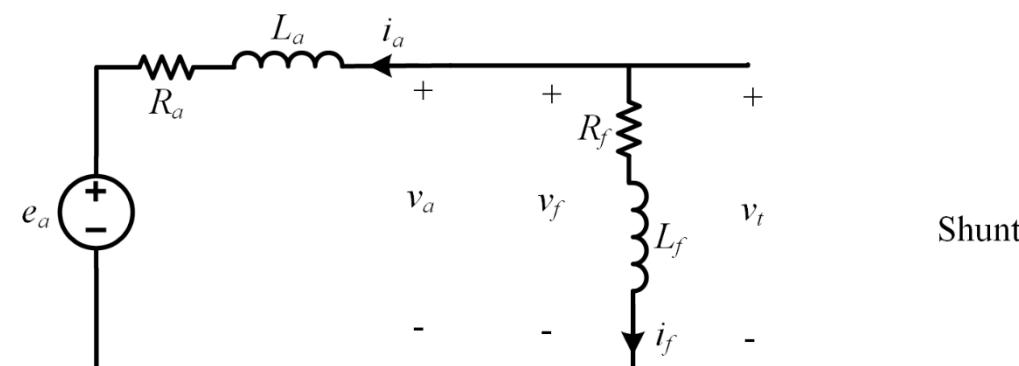
$$v_a = R_a i_a + e_a; \quad e_a = K\phi_f \omega_m \Rightarrow v_a = R_a i_a + K\phi_f \omega_m$$
